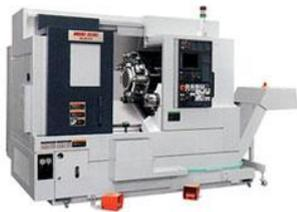
Gambar 2. Mesin CNC Lathe (Mesin Bubut)
